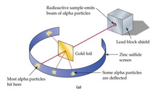
After the experiment had been set up in accordance to the speculations described above, Rutherford would fire the beam of alpha particles through the piece of foil and observe the location at which the particles landed on the screen.
